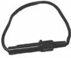
FS45350** FS45352 (Bulk 100pcs./carton) FUSE HOLDER • Black plastic twist lock case • 8" - 14 gauge wire loop • Includes 20 amp SFE fuse
