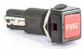
FS22080** FS22082 (Bulk 100pcs./carton) FUSE HOLDER • Panel mount with red fuse label • For glass fuses up to 20 amp • For panels up to 5/16" thick
