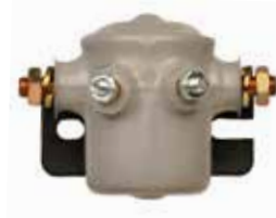
BA58010 SOLENOID SWITCH • Weather resistant plastic coating • Composite mounting bracket • 12 V insulated • Rated 85 A continuous duty
