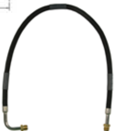
18-8114 FUEL LINE HOSE UNIVERSAL For fuel pump to carburetor connection. Replaces copper or steel tubing 3/8" X 31" PTFE composite hose with 5/8"-18 male inverted flare straight one end, 5/8"-18 90° one end. SAE J1527 type A1
