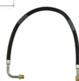
18-8115 FUEL LINE HOSE UNIVERSAL For fuel pump to carburetor connection. Replaces copper or steel tubing 3/8" X 25" PTFE composite hose with 5/8"-18 male inverted flare straight one end, 5/8"-18 90° one end. SAE J1527 type A1
