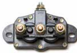
BA58020 • Motor reversing • Dynamic braking when both coils are in same electrical state • 12/24V DC • Intermittent rating: 150A • Continuous rating: 75 amp (5 min.)
