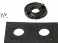
MP78960 MP78962 (BULK 100 PCS/CTN) Anti-rotation collar. Use when installing non-illuminated RotoSwitches in very thin dash panels. This adapter prevents the switch from "slipping" if excessive force is used to actuate the switch.
