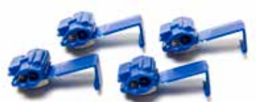
TC43904 Non-Strip Splicers Four blue non-strip splice connectors for making secure, permanent splices without stripping wires manually. Crimp with pliers and metal insert makes connection. Plastic top folds over to insulate connection.
