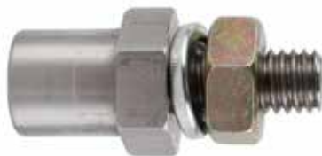
18-8412 STARTER STUD EXTENDER Extends the solenoid stud on PMGR starters for applications that require more accessory wire connections. Threads: Female M8x1.25, Male 3/8"x16 UNC
