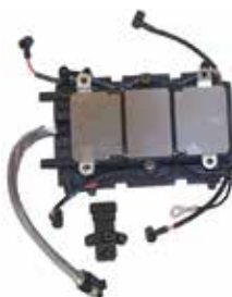
18-5886 POWER PACK & SENSOR Replaces: 436367, 584122 For: V6 engines with optical sensor and BLUE sleeve on power pack. Do not use with gray sleeved stator.
