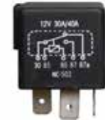
18-5705 POWER TRIM/FUEL PUMP RELAY Replaces: 582472, 584416, 586224 5 Terminal Single Pull - Double Throw - 12 Volt Open Contact: 40 Amps Resistive 30 Amps Conductive Closed Contact: 20 Amps Resistive 15 Amps Conductive
