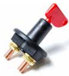
UN77310** BATTERY SWITCH Polyester housing is rust and corrosion proof. Removable plastic key for security. Two position switch "Off-On". Two 10MM X 1.5MM stud terminals. For panels up to 1.25 thick. Four mounting holes in a rectangle 1.3" and .8" on centers. 350 amp continuous rating. 500 amp intermittent rating.
