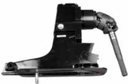
18-2419 COMPLETE UPPER GEAR CASE Replaces: 1547-9412A21, 1547-3917A4, 1547-3917A8, 1547-3917A16, 1547-3917A30, 1547-3917A38, 1547-5523A8, 1547-5523A11, 1547-8265A16 For: Alpha I 1.65:1/1.62:1
