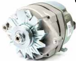
18-5957 ALTERNATOR Replaces: 3860769 (3-Wire) (68 AMP) Replaces Mando, Motorola and Original Equipment Delco. Uses same electrical connections and mounting method. Equipped with fan and drive pulley. SAEJ1171
