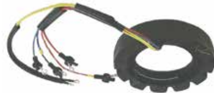
18-5859 STATOR Replaces: 398-5454A26, 398-5454A22, 398-5919A7, 398-5919A3
