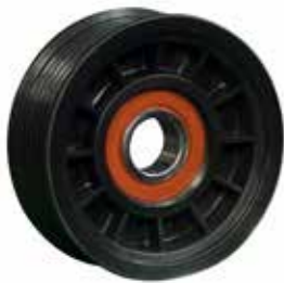
18-6457 COMPOSITE PULLEY Replaces: 807757T 3" OD Serpentine for 13/16" width belt For: Late model GM V6 & V8 engines
