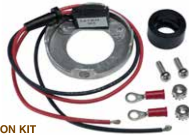
18-5299D Display Package 18-5299 ELECTRONIC CONVERSION KIT With screw down cap For: Most Prestolite V-8 Distributors Use with 18-5403 style rotor
