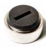
MP39270** FACENUT For polyester ignition switches MP39100 thru MP39120. Nut has extra long threads for positive engagement on mounting bushing for early (Pre-1995) style with 13/16"-20 thread ONLY!
