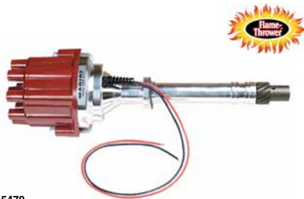
18-5479 ELECTRONIC DISTRIBUTOR GM V-8 engines-reverse rotation Replacement Cap/Rotor Kit 18-5266
