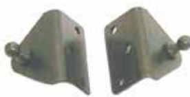
GS62880 Black zinc plated steel 90° angle bracket with 10mm ball stud. 2" x 1.2" base
