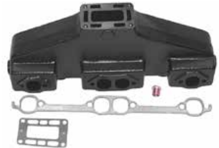
18-1898 MANIFOLD Port & Starboard Replaces: Barr CHVA-1-84, Marine Power 0991-110 Fits 454 cu.in. GM big block V8 engines Use with: Exhaust Manifold Gasket: 18-0418 *For Exploded View - See Pages 636-637
