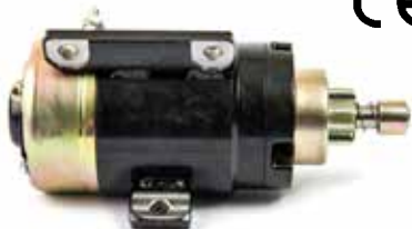
18-6423 OUTBOARD STARTER Replaces: 688-81800-12-00 Fits: C75 (1994-96), (1998-99), P75 (1996-99), C80 TLRV (1997), C85 (1991-96) CV85 (1990), 90 (1984-03), B90 (1998-99) C90 (1997-01)
