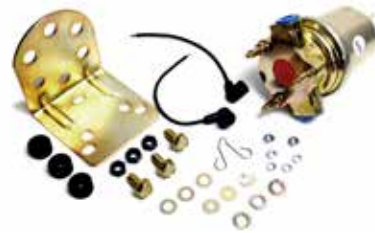
18-7333 ELECTRIC FUEL PUMP UNIVERSAL 12V, 72GPH at 5.75 PSI, 1/4" NPSF for 3/8" hose, for use with gasoline and diesel fuel. OP72533 pressure safety switch recommended.
